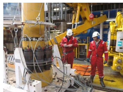
A WellPartner HP-Riser flange about to be made-up with special tooling on the drill floor of a NCS jack-up rig.
