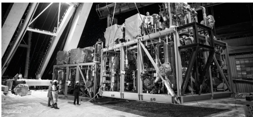
Minox Compact deaeration package ready for transport from Agility Subsea Fabrication in Langesund, Norway to Hebron offshore Canada.
