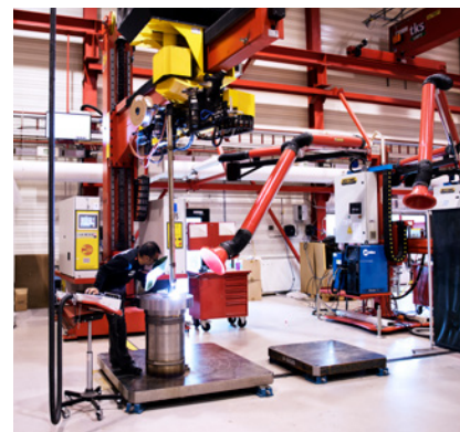
Welding of a subsea component at Aarbakke's modern factory at Bryne.
