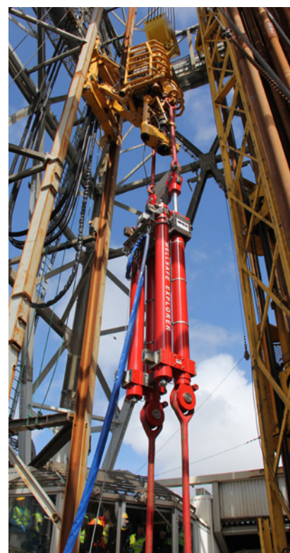
The WellSafe Explorer from WellPartner is designed to protect people, environment and equipment. It is a safety element in subsea well access systems for semi-submersible drilling rigs and drillships during live well operations.
