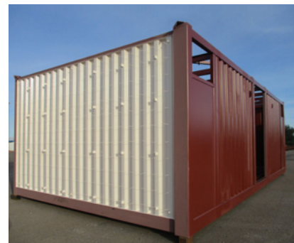
A welded and painted module ready for outfitting.
