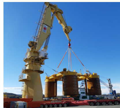
Large structure mobilization enabled by 400 ton AHC crane.
